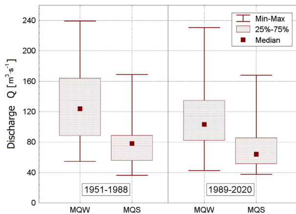
Fig. 14. Range of variability of the seasonal discharge of the Warta River in Poznań in sub-periods 1951–1988 and 1989–2020. MQW, average discharge in the cold half-year (November–April; unit: \text{m}^3 \cdot \text{s}^{-1} ); MQS, average discharge in the warm half-year (May–October; unit: \text{m}^3 \cdot \text{s}^{-1} ).
