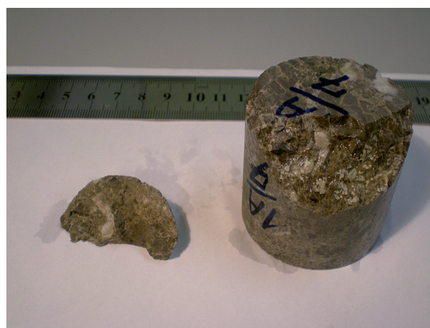
Fig. 8. Fragments fallen off sample 1/7 after 149 gelation cycles
