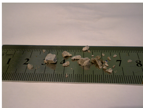
Fig. 8. Fragments fallen off sample 1/7 after 149 gelation cycles
