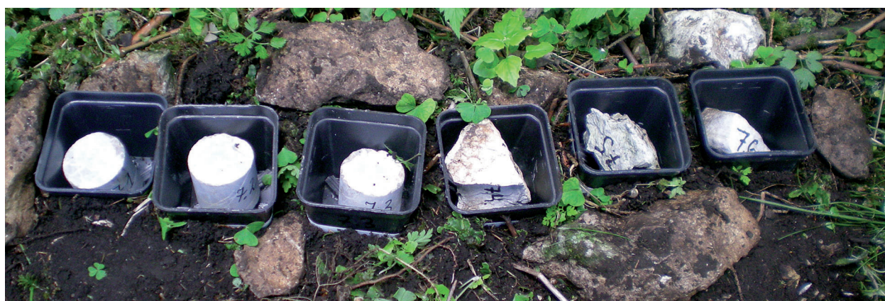
Fig. 4. Field experiment: measurement of weathering rates in natural conditions
