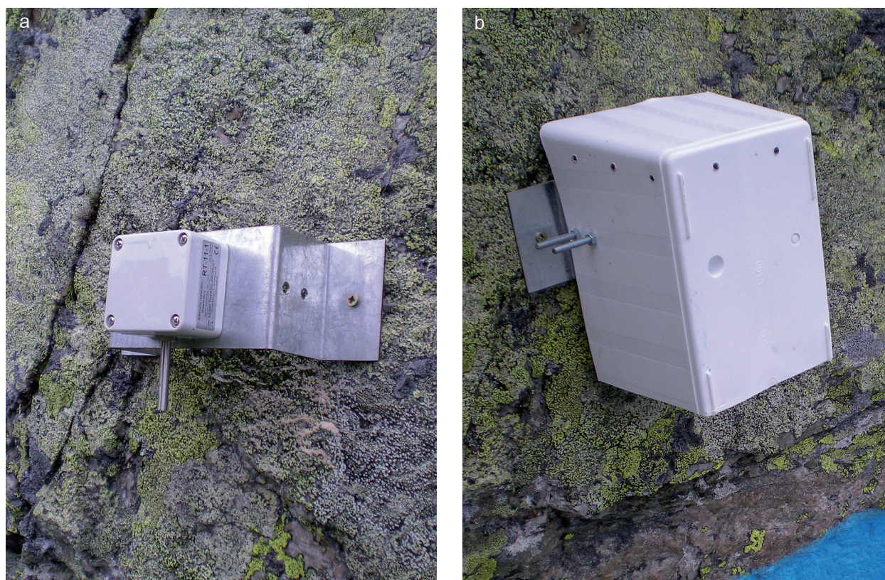
Fig. 5. Temperature recorders a) unshielded; b) shielded from sunlight
