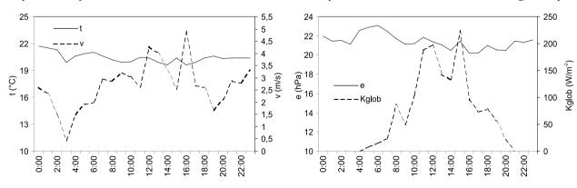
Fig. 18. Daily course of air temperature (t), wind speed (v), water vapour pressure (e) and total solar radiation (Kglob) in Łeba on 23rd July 2010.
